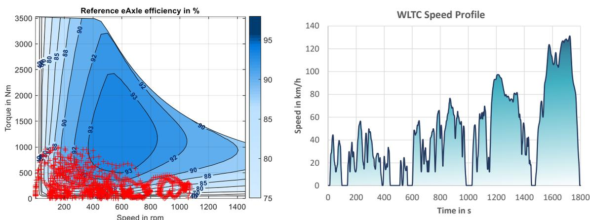
Figure 4: WLTC speed profile and resulting torque-speed points for a reference C-segment EV<sup>3</sup> in the operating area of an eAxle
