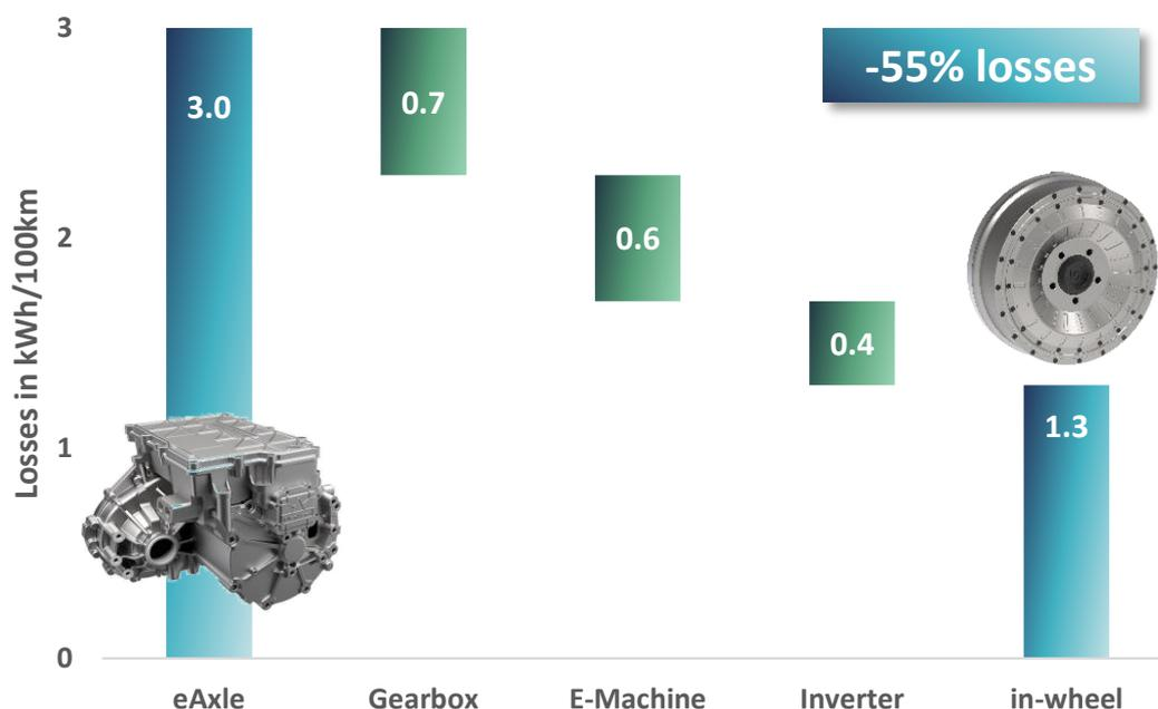
Figure 6: Loss reduction of the DeepDrive in-wheel motor compared to the generic eAxle at nominal temperature (60°C). For low temperature (10°C) operation, the loss reduction rises to 2.5 kWh or 65%. The inserted picture of the eAxle (Source: BorgWarner<sup>7</sup>) is just for illustrative purpose.
