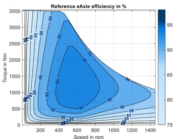
Figure 3: Specifications of generic reference eAxle and resulting efficiency map based on own calculation
