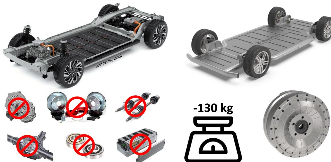
Figure 7: Removed components and weight savings in DeepDrive platform with in-wheel motors compared to conventional EV-platforms
